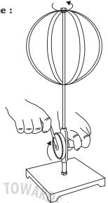
**Step 1:** Insert assembly 'b' in the drilling machine of assembly 'a'. Fix it with screw provided at the end of assembly 'b'. Now rotate the drill machine by using its handle as fast as possible. Simultaneously notice the change in the shape of the circular loops of elastic steel strips. They take a elliptical shape as they execute circular motion.
